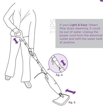
2 Wait 30 seconds for the boiler to heat the water. Pump the handle a few times to prime the pump, activate steam and moisten the micro-fiber pad. (fig. 4)
